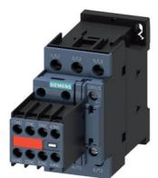
power contactor, AC-3e/AC-3, 9 A, 4 kW / 400 V, 3-pole, 230 V AC, 50/60 Hz, auxiliary contacts: 2 NO + 2 NC, screw terminal, size: S0, captive auxiliary switch
