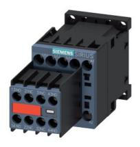
power contactor, AC-3e/AC-3, 9 A, 4 kW / 400 V, 3-pole, 230 V AC, 50/60 Hz, auxiliary contacts: 2 NO + 2 NC, screw terminal, size: S00, captive auxiliary switch
