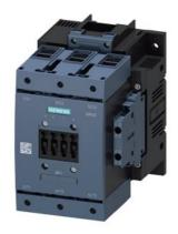
Power contactor, AC-3 115 A, 55 kW / 400 V AC (50-60 Hz) / DC operation 23-26 V UC Auxiliary contacts 2 NO + 2 NC 3-pole, Size S6 with box terminals Drive: conventional screw terminal
