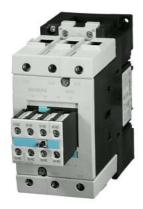
Power contactor, AC-3 95 A, 45 kW / 400 V 230 V AC, 50 Hz, 2 NO + 2 NC 3-pole, Size S3 Screw terminal !!! Phased-out product !!! Successor is SIRIUS 3RT2 Preferred successor type is >>3RT2046-1AP04<<
